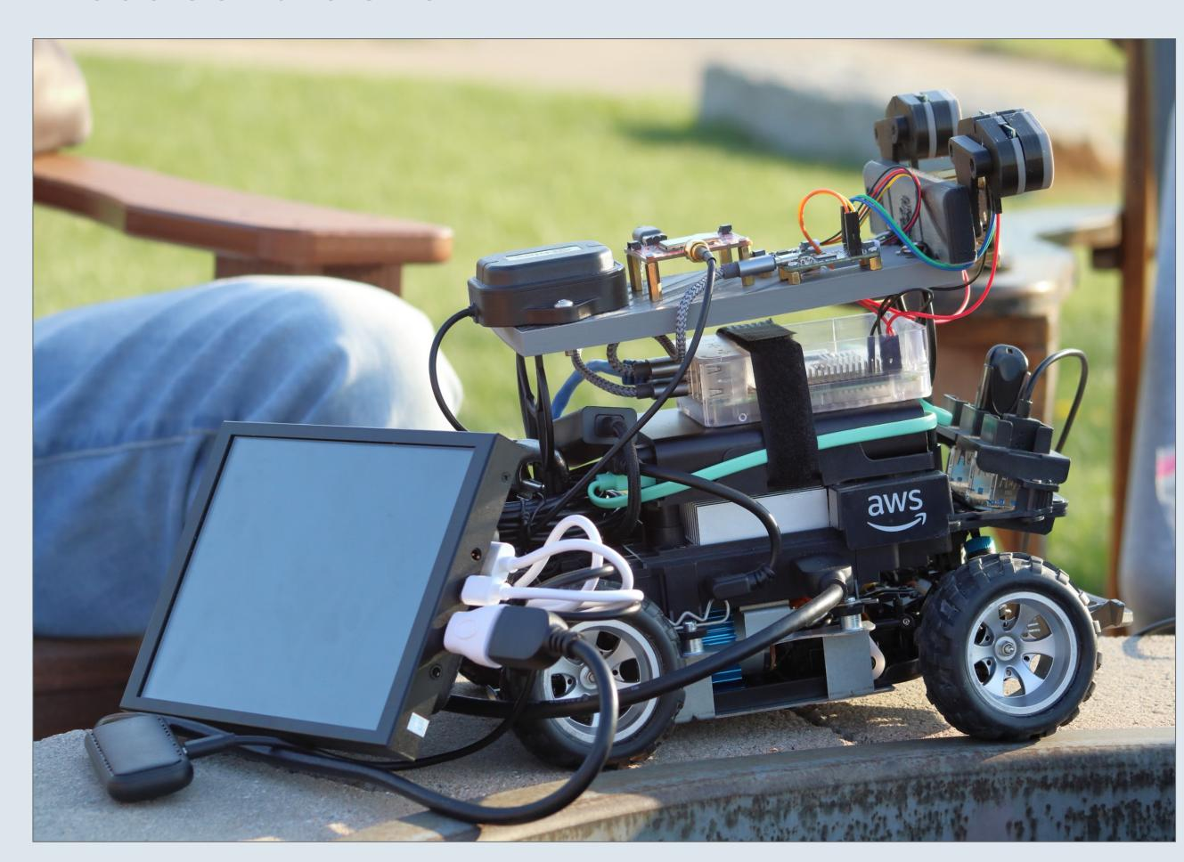
CADD-E implements the same perception and decision-making modules that would be used on a full-size autonomous vehicle. We performed on-site testing to verify our implementation.
